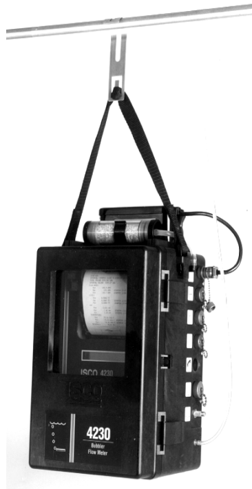
Figure 3-2 4230 Suspended by Handle (handles may vary)
