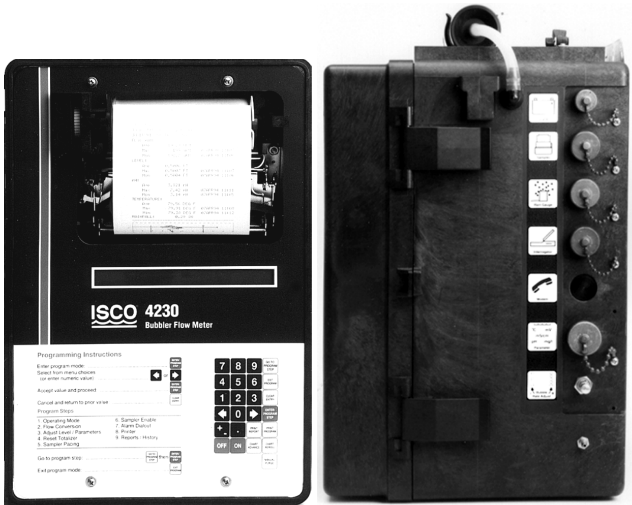
Figure 1-2 4230 Controls and Indicators (left), Connectors (right)
