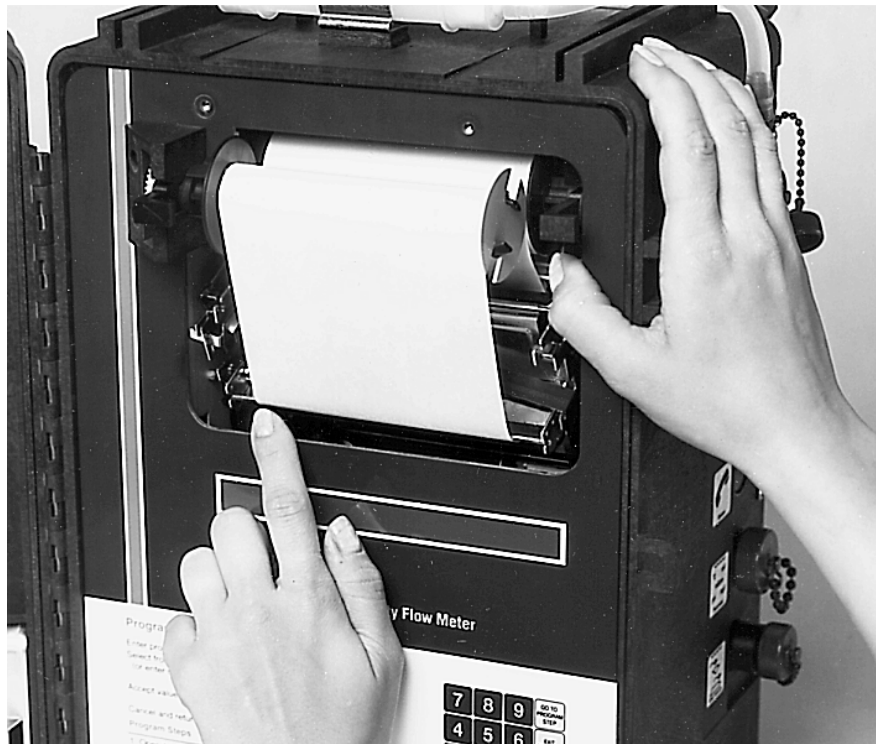
Figure 5-4 Lifting the Flow Meter from the Case
