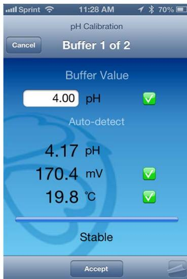
6. Fill the cup to the fill line with the second calibration buffer. Place the instrument into the calibration cup, and tap **Start**.
