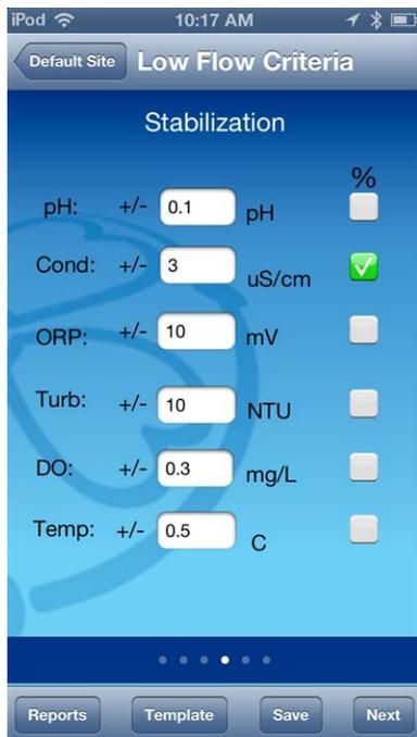
10. A green checkmark indicates that the stabilization criterion for the parameter is based on percentage rather than an absolute value. Tap a gray box to change from absolute to percentage.
