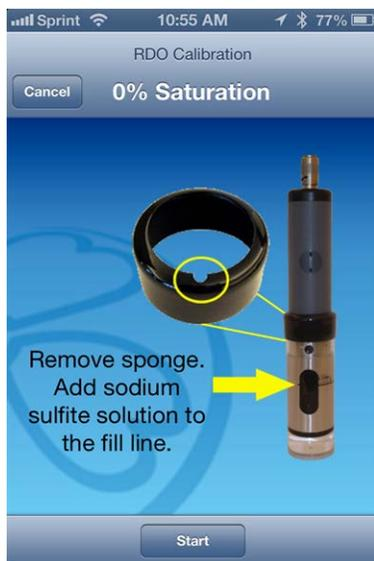
7. When the calibration is stable, tap the **Accept** button.
