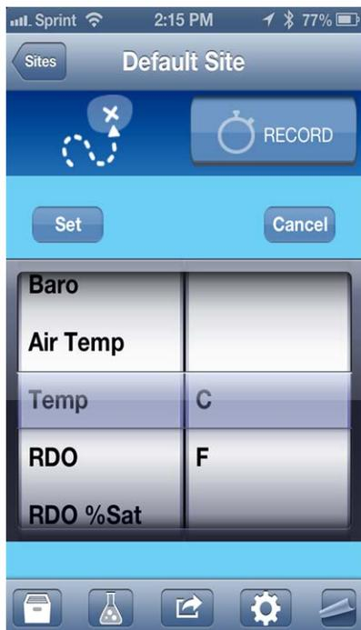
2. Swipe the left side of the parameter pick wheel to find the appropriate parameter.
