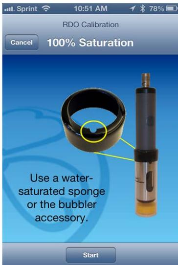
5. When the calibration is stable, tap the **Accept** button.
