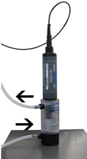
1. Select the barbed NPT fitting that will fit with the tubing size.
