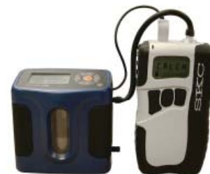
Multiple-point calibration train with CalChek; do not place sample medium in line.
