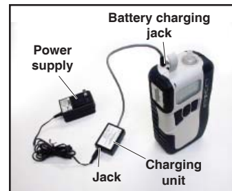
Leland Legacy charging train with single charger
