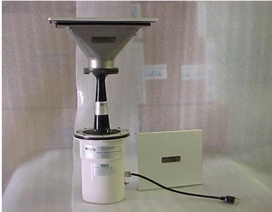
TE-10557 PM10-BL Brushless Volumetric Flow Controller w/Look Up Table. Controls a Constant Flow through, 8" x 10' Filter Media (TE-QMA Micro Quartz Filter Media required or PM10). See Photo Below
