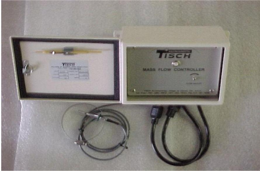
TE-300-310-BL Brush-less Mass Flow Controller with 20 to 60 SCFM Air Flow Probe.
