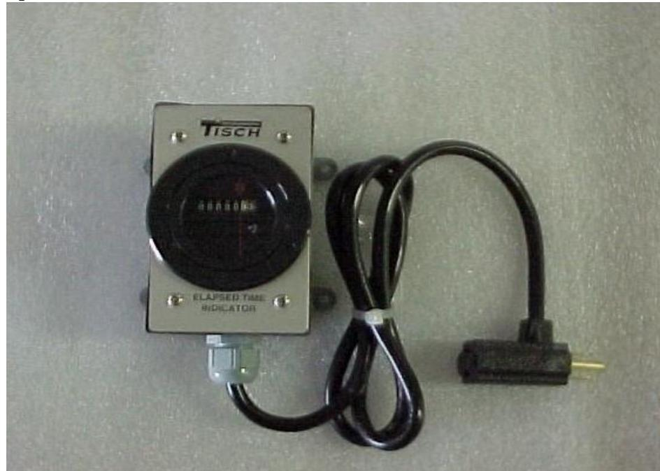
TE-5013 Elapsed Time Indicator Mechanical E.T.I. Registers how long the PM10 System ran 0000.0 minutes. Similar to TE-5012 ETI except this product features a re-settable clock.
