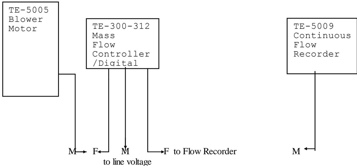
The TE-5005 Blower Motor male cord set plugs into the TE-300-312 Mass Flow Controller/ Digital Timer/ETI left Timed Female cord set.
