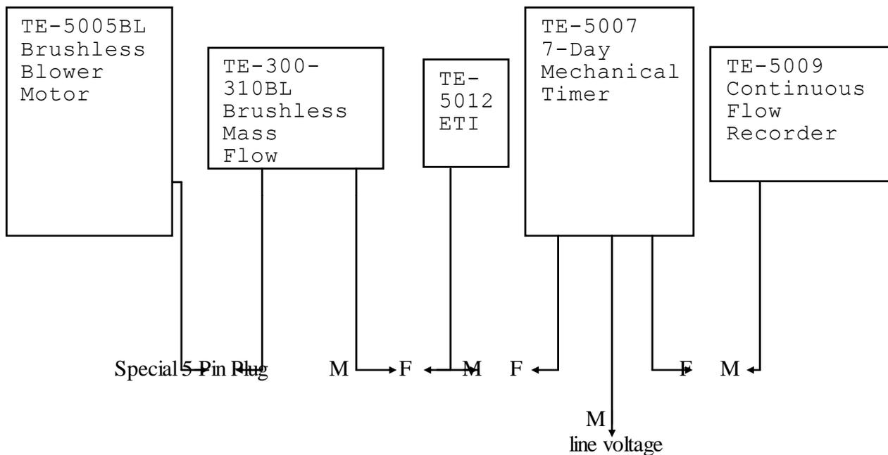
The TE-5005BL Brushless Blower Motor special 5 pin male cord set plugs into the special 5 pin female cord set on the TE-300-310BL Brushless Mass Flow Controller.
