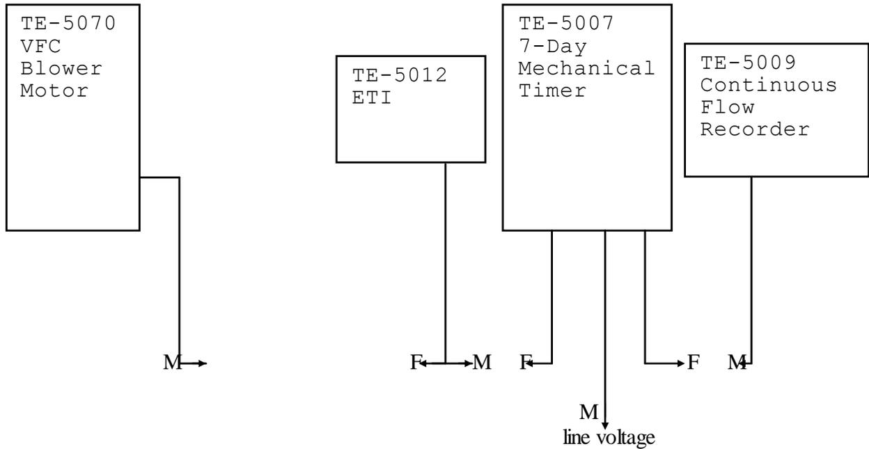
The TE-5070 VFC Blower Motor male cord set plugs into the TE-5012 Elapsed Time Indicator female side.
