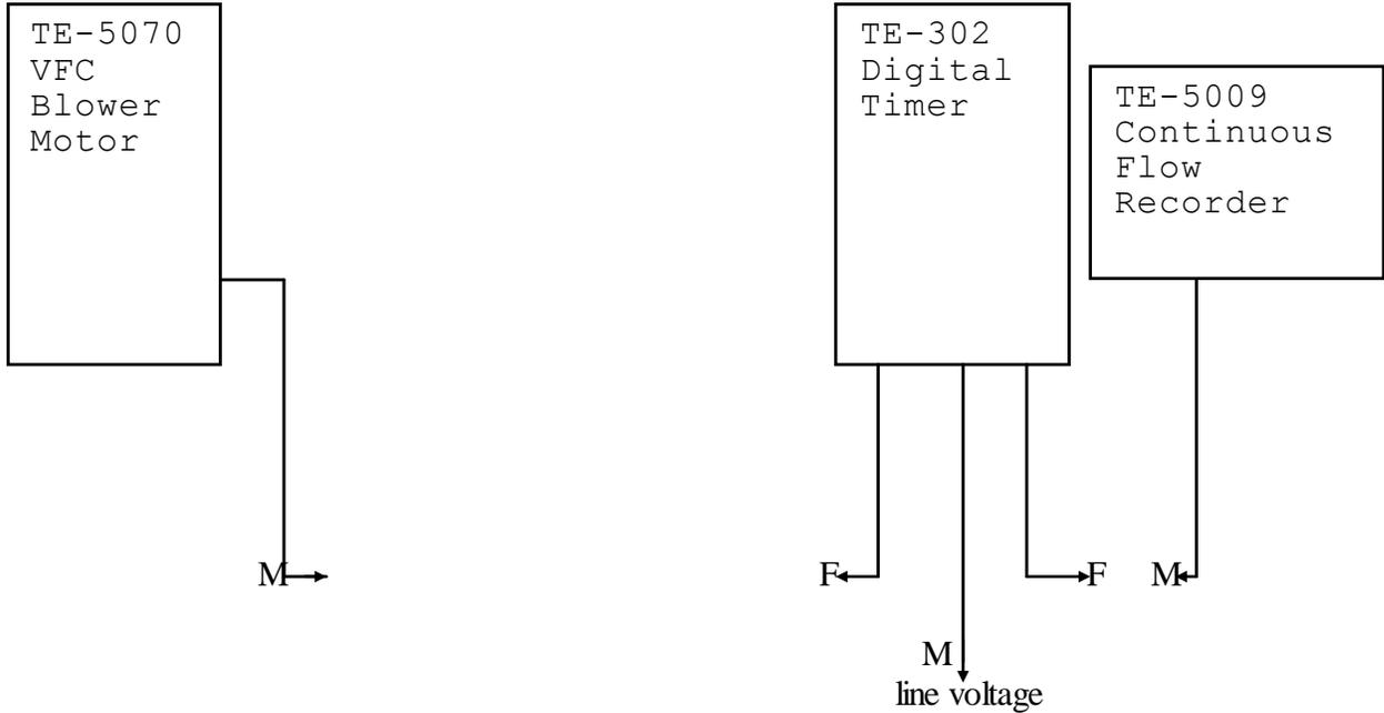
The TE-5070 VFC Blower Motor male cord set plugs into the TE-302 Digital Timer timed female cord set which is on the left side of timer.
