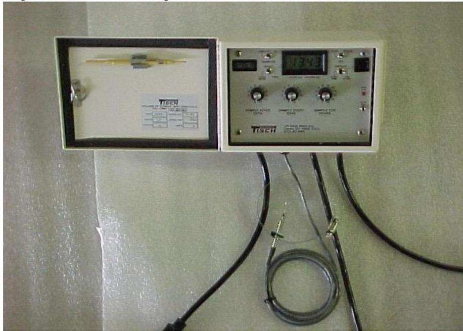
TE-10557 PM10 Volumetric Flow Controller w/Look Up Table. Controls a Constant Flow through, 8" x 10' Filter Media (TE-QMA Micro Quartz Filter Media required for PM10). See Photo Below.
