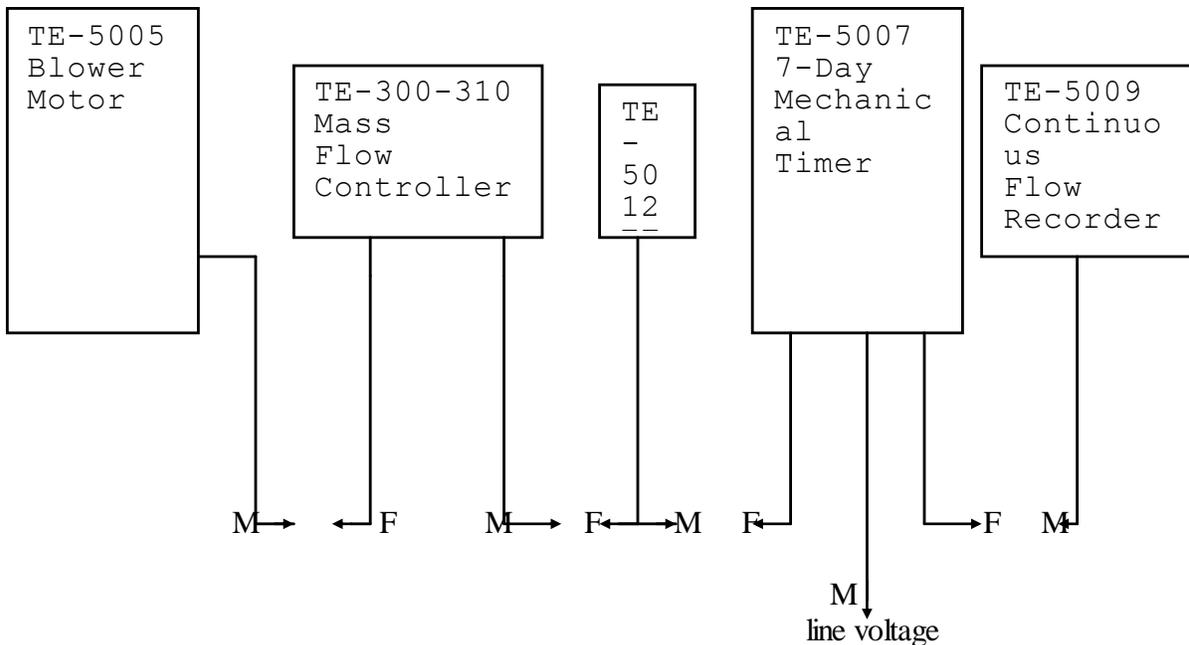
The TE-5005 Blower Motor male cord set plugs into the TE-300-310 Mass Flow Controller Female cord set.
