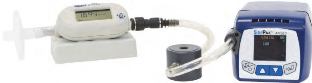
TSI 4146 flow meter (sold separately) being used to calibrate flow setting for AM520
