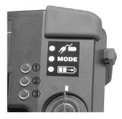
The status LEDs indicate the device status of the flue gas analyzer:
