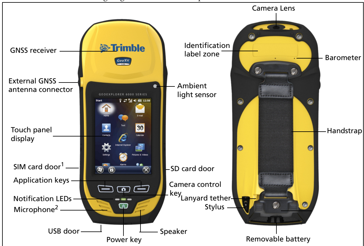
Figure 2.1 Parts of the GeoExplorer 6000 series handheld
