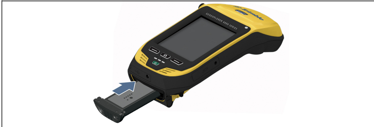
Figure 2.1 Inserting the battery
